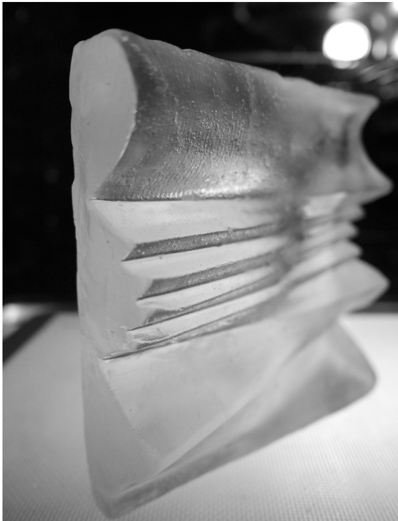
Figure 11: A detail image of a completed glass block resulting from the analog design to robotic fabrication workflow.
